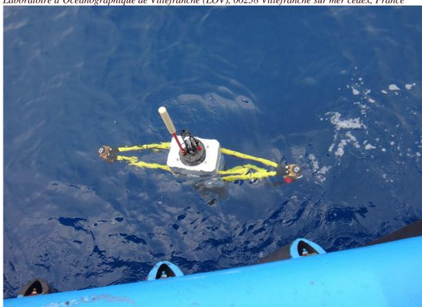
A ProVal profiling float, which is dedicated to the validation of satellite ocean color remote sensing data, was deployed at the BOUSSOLE site, from the deck of the R/V *Téthys II*.
